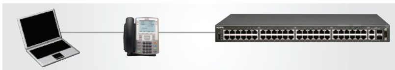
Figure 1. Typical enterprise converged connectivity
